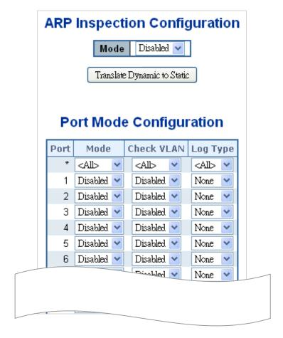
Figure 4-5-9-1: ARP Inspection Configuration Screen Page Screenshot
