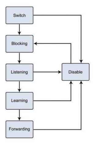
Figure 4-3-9-1: STP Port State Transitions
