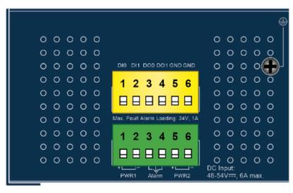
Figure 2-12: IGS-5225-8P2T2S, IGS-5225-8P2T4S, IGS-5225-8P4S and IGS-5225-8P4S-12V Upper Panel
