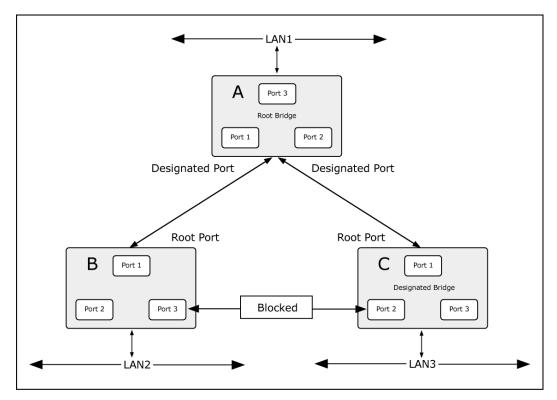
Figure 4-3-9-3: After Applying the STA Rules
