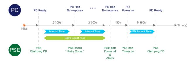
This page provides you how to configure PD Alive Check. The screen in Figure 4-6-1-7 appears.
