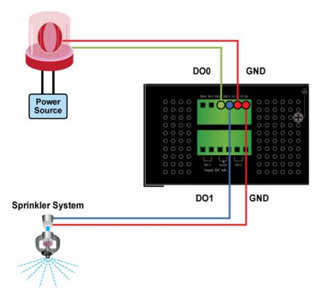
Figure 2-20: Wiring DO0 and DO1 to Open Detector
