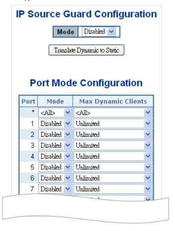
Figure 4-5-7-1: IP Source Guard Configuration Screen Page Screenshot
