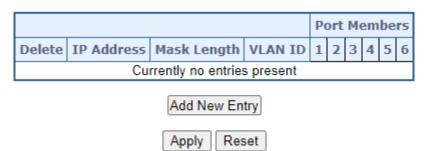
Figure 4-3-6-2: IP Subnet-based VLAN Membership Configuration
