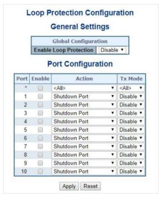
Figure 4-3-15-1: Loop Protection Configuration Page Screenshot
