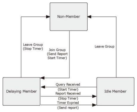
Figure 4-3-10-4: IGMP State Transitions
