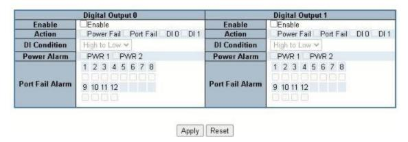
Figure 4-2-20 Digital Output Control Configuration page Screenshot
