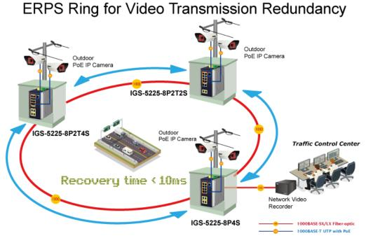
Figure 4-8-1: Ring Example Diagram
