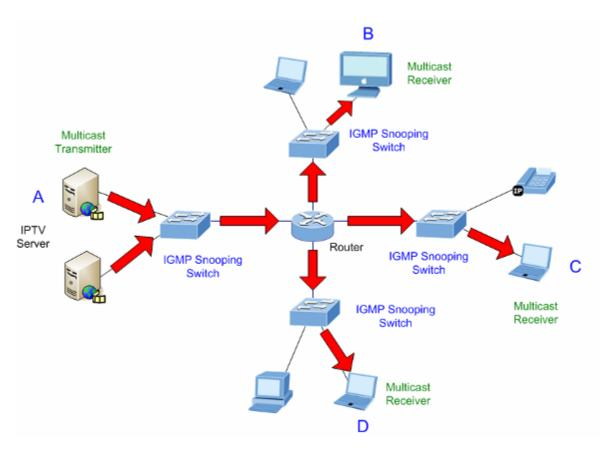
Figure 4-3-10-3: IGMP Snooping Multicast Stream Control
