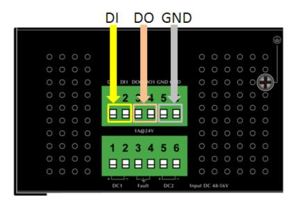
Figure 2-17: Wiring the Redundant Power Inputs
