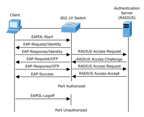
Figure 4-5-2-2: EAP Message Exchange
