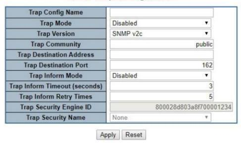
Figure 4-2-2-4: SNMP Trap Configuration Page Screenshot
