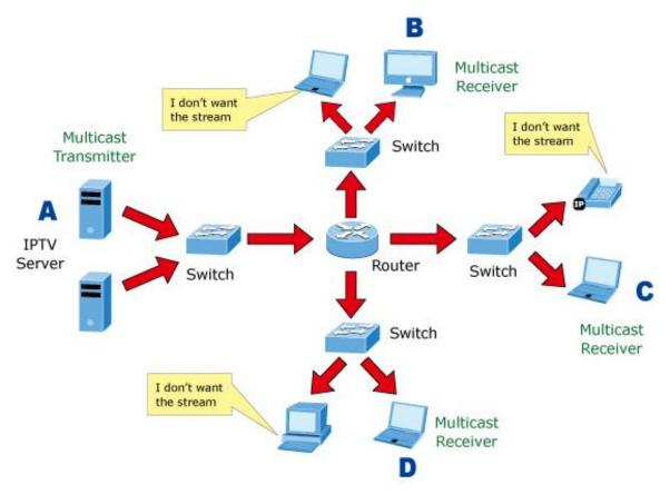
Figure 4-3-10-2: Multicast Flooding
