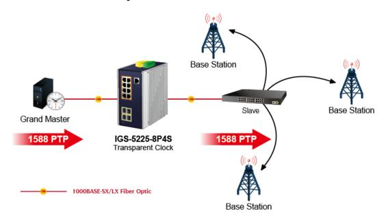
PTP was originally defined in the **IEEE 1588-2002** standard, officially entitled "Standard for a Precision Clock Synchronization Protocol for Networked Measurement and Control Systems" and published in 2002. In 2008 a revised standard, **IEEE 588-2008** was released. This new version, also known as PTP Version 2, improves accuracy, precision and robustness but is not backwards compatible with the original 2002 version.
