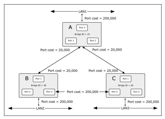
Figure 4-3-9-2: Before Applying the STA Rules
