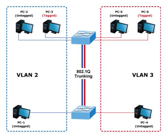
Figure 4-3-3-11: VLAN Trunking Diagram
